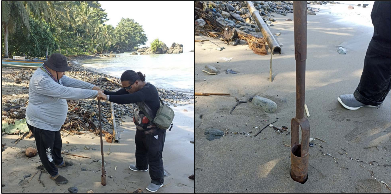
Figure 2. Coastal sediment sampling with hand auger
